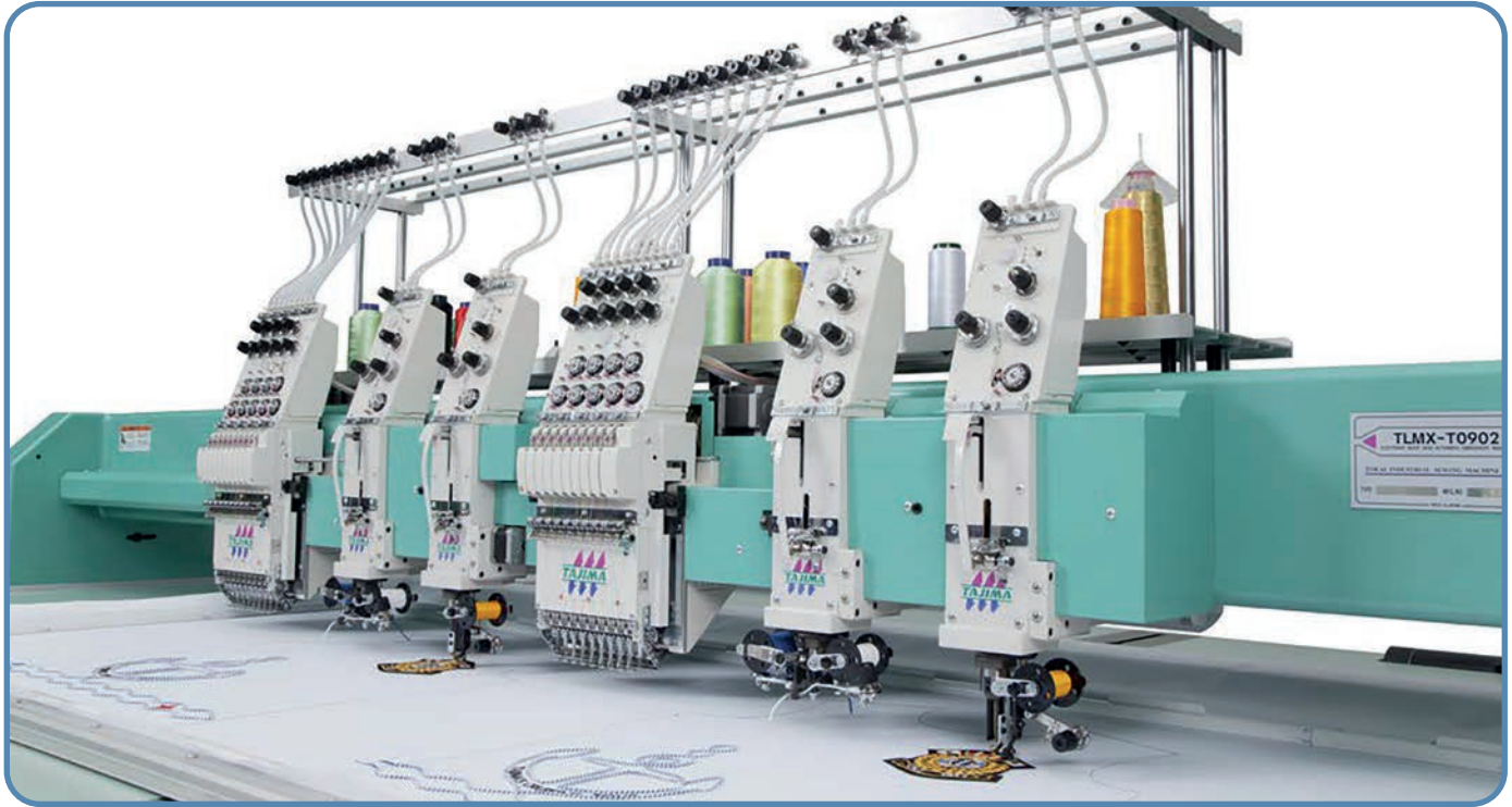
TLMX TRIPLE MIXED TYPE MACHINE: 2 LOCK STITCH CHENILLE + 1 MULTI COLOR HEAD
